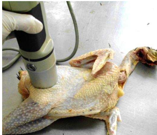
Fot. 6. Pomiar barwy tuszki Z-11 aparatem Minolta w skali L^*a^*b^* Fig. 6. Measurement of L^*a^*b^* colour values of Z-11 carcass with a Minolta device
